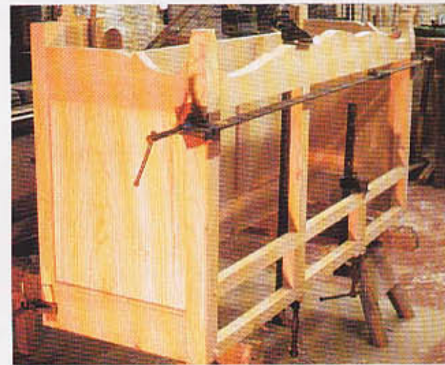
Once glued, I immediately fitted the 18mm plywood floor to give it rigidity
