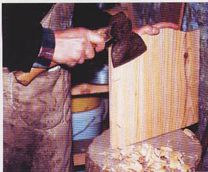
A sharp axe is probably no slower than using a hand held planer, and much quieter
